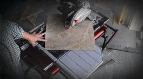
ackmond Products, Inc., a leading supplier of diamond tools, carbide tools and equipment, recently created a joint venture with Delta designing a new 7-inch wet tile saw. The Beast7, 7-inch tile saw offers virtually the largest rip and diagonal cutting capacity in its class. It is capable of performing a diagonal cut on a 18- x 18-inch tile, and it can execute a 24-inch rip cut.
