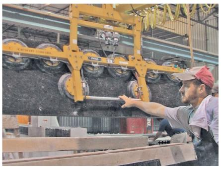
A vacuum lifter is in place to move slabs safely around the workspace.
